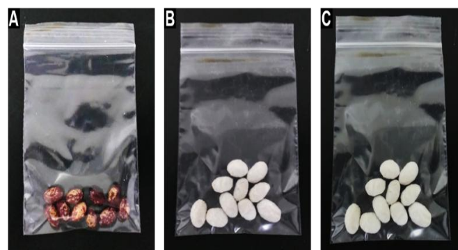
Figure 2. Treatment of Phaseolus vulgaris L var. José Beta seeds. (A) Seeds of Phaseolus vulgaris L var. José Beta uncoated. (B) Seeds of Phaseolus vulgaris L var. José Beta coated with PEO nanofibers. (C) Seeds of Phaseolus vulgaris L var. José Beta coated with PEO nanofibers that have the AMF inoculant incorporated.
