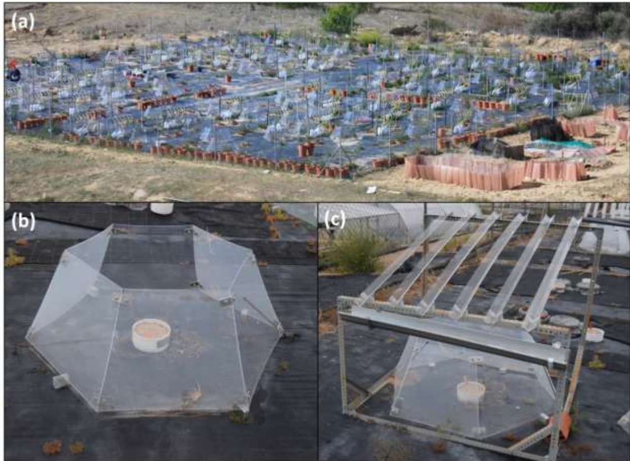
Fig. S2 View of the experimental site (a) and details of simulated climate change treatments: warming, consisting of OTC (b), and the combination of warming and reduced precipitation, consisting of OTC + rainfall shelter (c). The OTCs were built with six methacrylate plates that followed a hexagonal design with sloping sides of 65-52-42 cm (b). The methacrylate material used to build them transmits ~92% of the visible spectrum, has a 4% of the emission of the infrared wavelength and pass on 85% of incoming energy (data provided by the manufacturer, Decorplax Metacrilatos S.L., Madrid, Spain). Each rainfall shelter has an area of 1.68 m 2 (1.4 m × 1.2 m), and a mean height of 1 m, and a roof composed of six methacrylate grooves (c), which covers approximately 35% of the surface.
